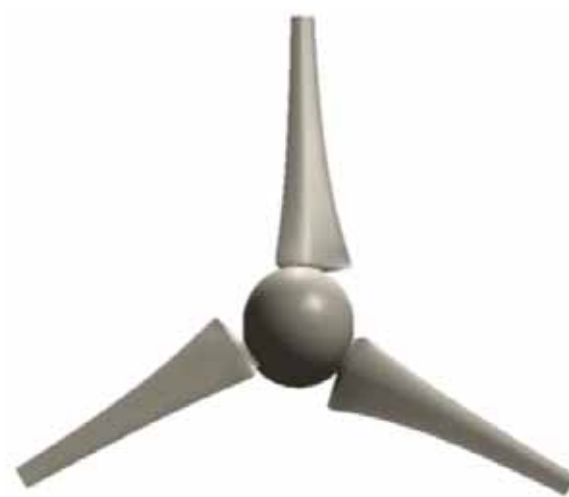
Fig. 6. 3D representation of the designed wind turbine rotor
